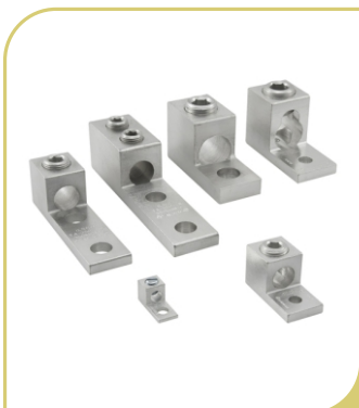
ILSCO Mechanical Lug, One Conductor, Mechanical connection, Dual Rated, Aluminum material, Tin plated connector, 1 mounting hole(s), mounting bolt/stud size 1/4 in, UL 486A/B Listed, UL 467 Listed, C22.2 No.
